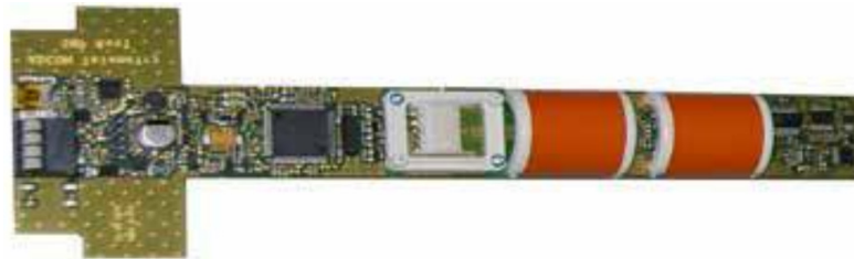
Fig. 3. Section of a soil parameter measuring probe
